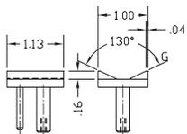
"V" block screw controlled backstop
