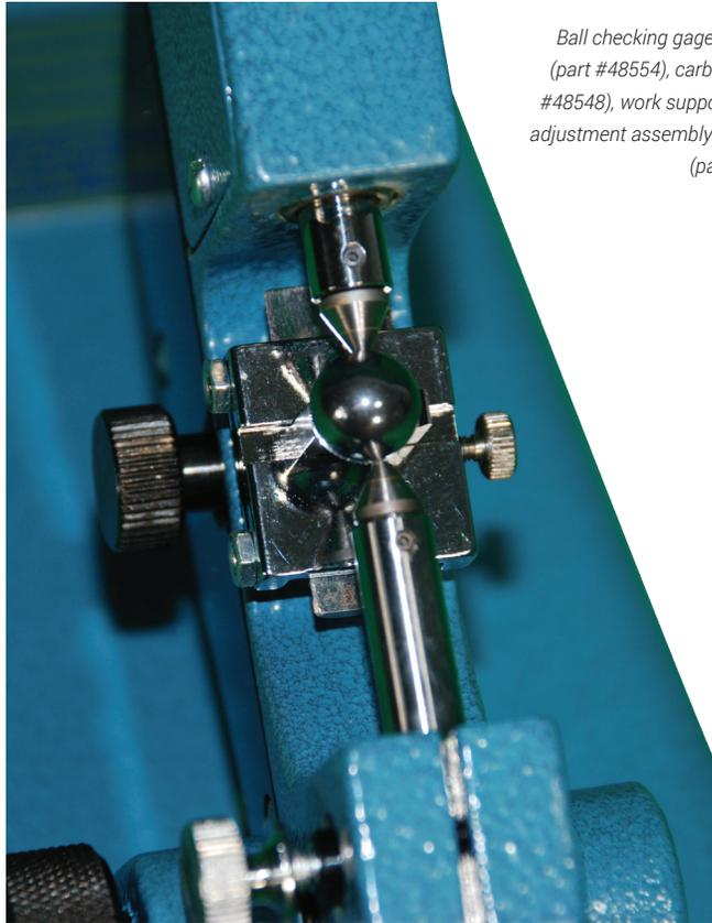
Ball checking gage shown is comprised of gage (part #48554), carbide tapered flat contacts (part #48548), work support (part #48569), work support adjustment assembly (part #48581), and bench stand (part #48502-V)
