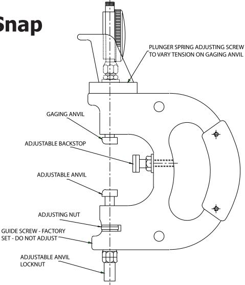
This gage has an adjusting range of 1" and is furnished with a Box Wrench for the Locknut. To set the gage to the Master, loosen Locknut with the Box Wrench and move Adjustable Pin by turning the knurled Adjusting Nut until Indicator Hand moves a little more than a quarter turn from rest position when gage is on master.
